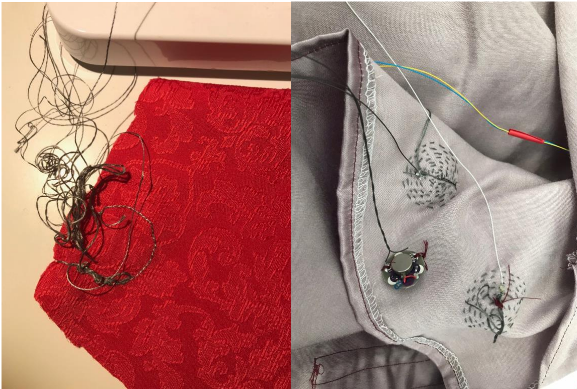
Figure 20: Testing conductive thread with sewing machine on left and haptic motor with conductive thread on right.
