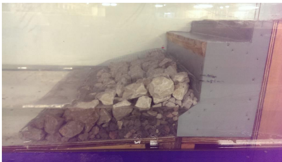
Figure 2: Modified sea wall model
