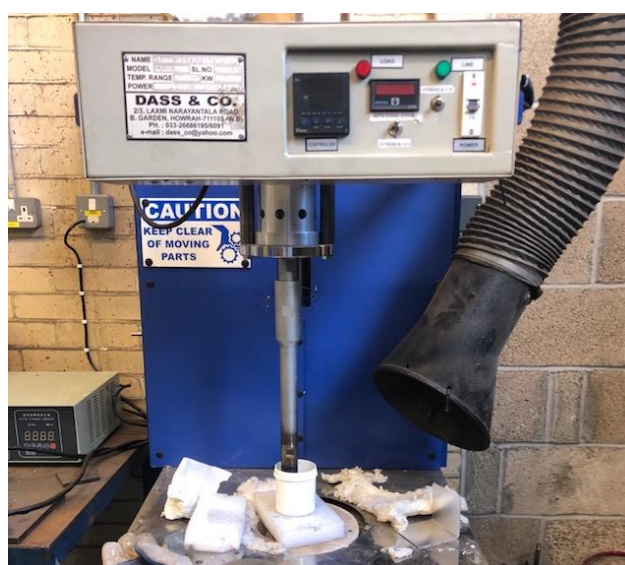
Figure 5: Ultrasonicator dispersing CNT/PDMS.
