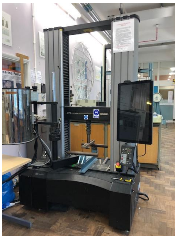
Figure 1: Instron 5582 used for tensile testing CT specimen.
