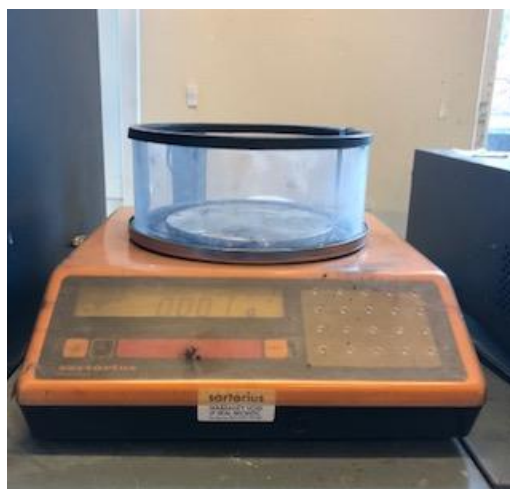
Figure 4: Sartorius scale for sample weight measuring.
