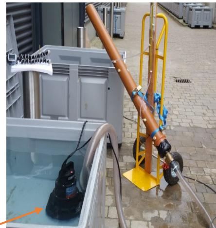
Figure-8: Submersible pump placed inside the tank to start pumping
