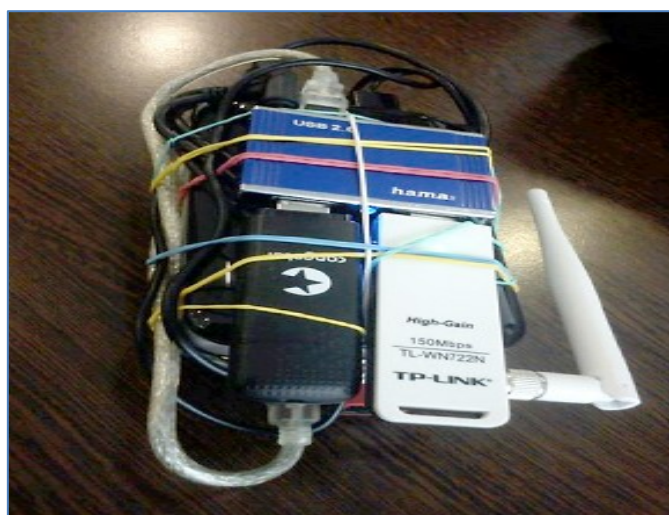
Figure 22: The components of portable Wi-Fi access point (F-Secure, 2014)
