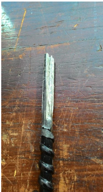
Photo 4 – BFRP Spiral Sanded Off at Each End. Test Failed by one end crushed.
