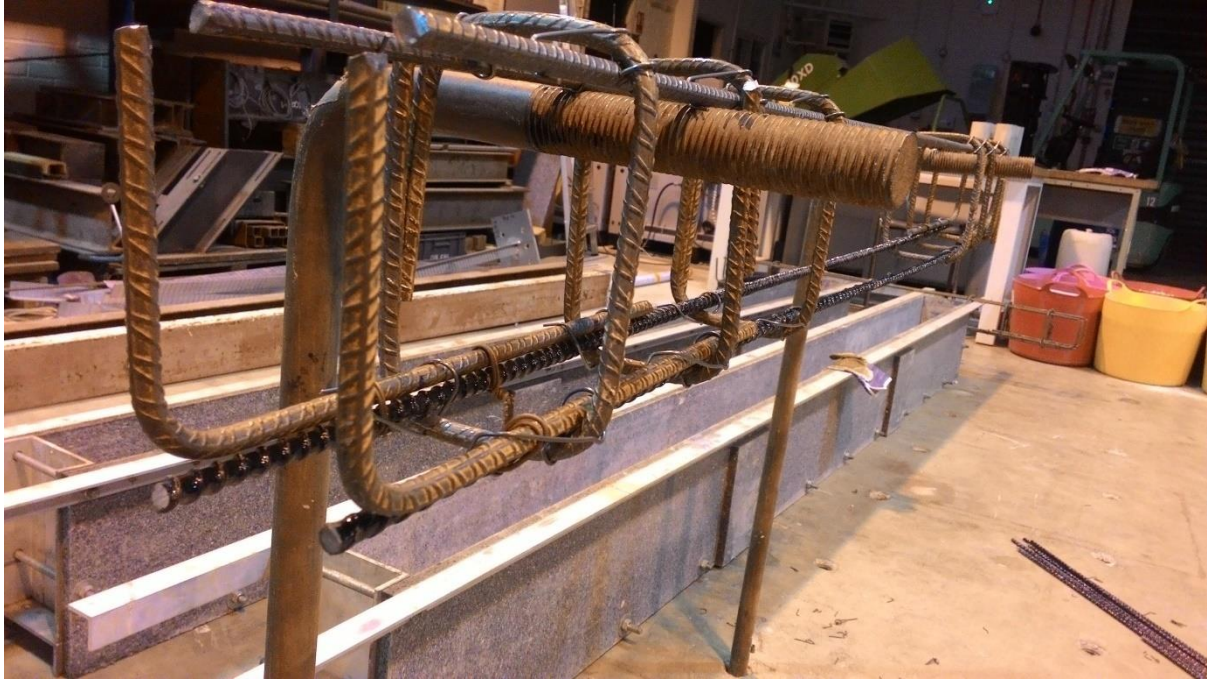
Photo 8 – BFRP and Steel Reinforcement Setup in Beams B2 and B4.
