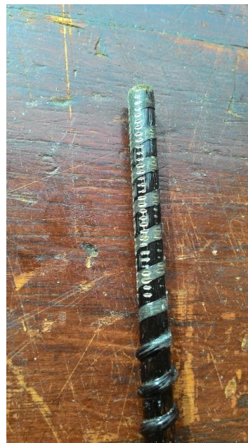
Photo 4 – BFRP Spiral Sanded Off at Each End. Test Failed by one end crushed.
