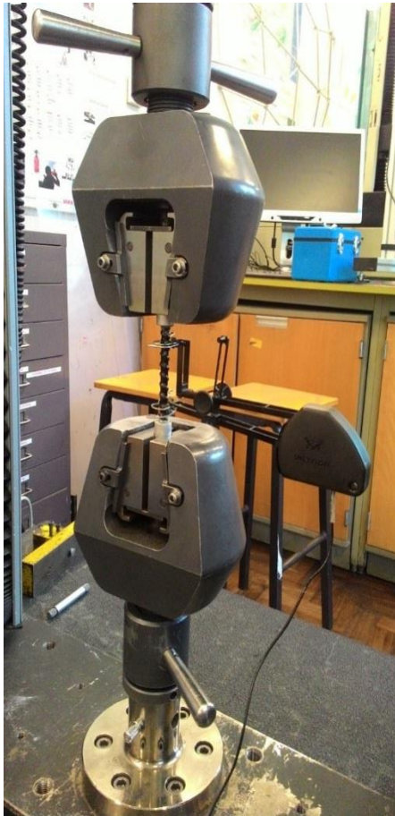
Photo 3 - Extensometer BFRP Rebar Inside The Testing Machine
