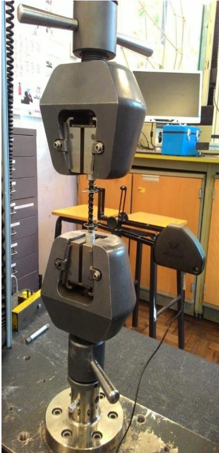
Photo 3 - Extensometer BFRP Rebar Inside The Testing Machine
