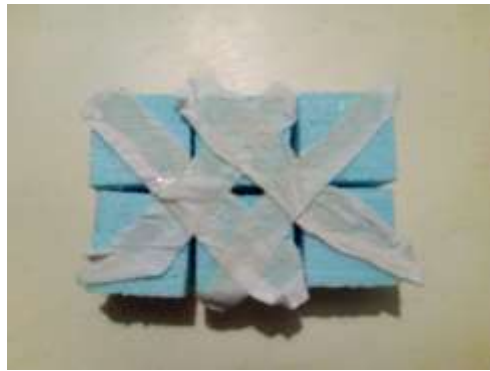
Figure 3.6 - Connection Method 2 - Diagonal Arrangement
