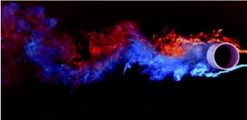
Figure 20 - Fluid turbulence shown using dye tracer (Tumbler, No date)
