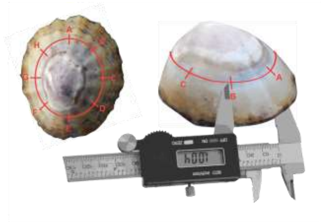
Figure 4: Left: top view of shell with demonstration of how 8 points (A-H) are marked around the centre of the shell – distance between each letter is equal. Right: indication of caliper use at one point. (Not to scale).
