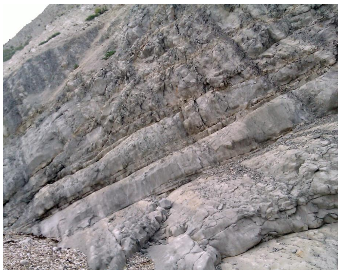
Figure 4.5 Discontinuities developed in the interbedded chalk and marls at Culver cliff. Notice that the discontinuities are running at nearly right angles to the bedding. This was also seen in the whiter Chalk succession seen after this.
