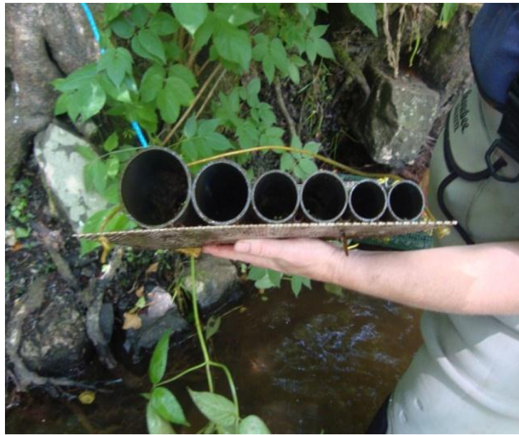
Plate 4. An example of an artificial refuge trap (ART) used in rivers.
