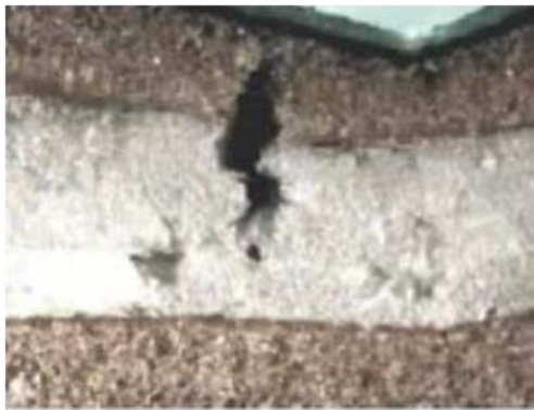
Figure 1.4: Crack propagating through foam after skin failure
