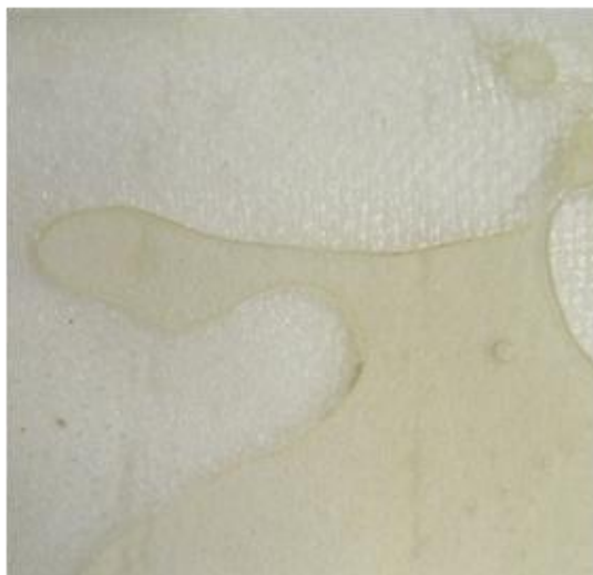
Figure 3.1: Area of excess resin on laminate.
