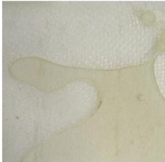
Figure 3.1: Area of excess resin on laminate.
