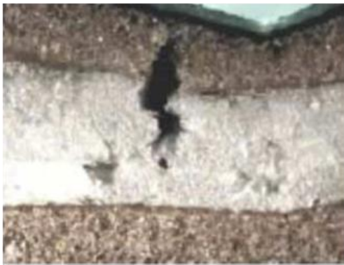
Figure 1.4: Crack propagating through foam after skin failure
