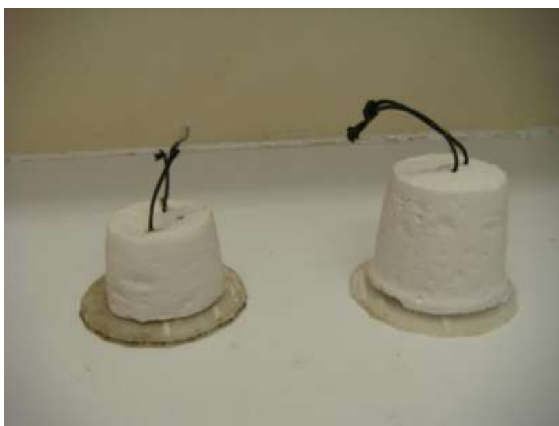
Plate 6. A plaster of Paris clod, hung at four regular intervals to measure the water flow at each marina. The clods above represent the contrasting marinas; even in the absence of scales the difference in water flow is clearly identifiable.
