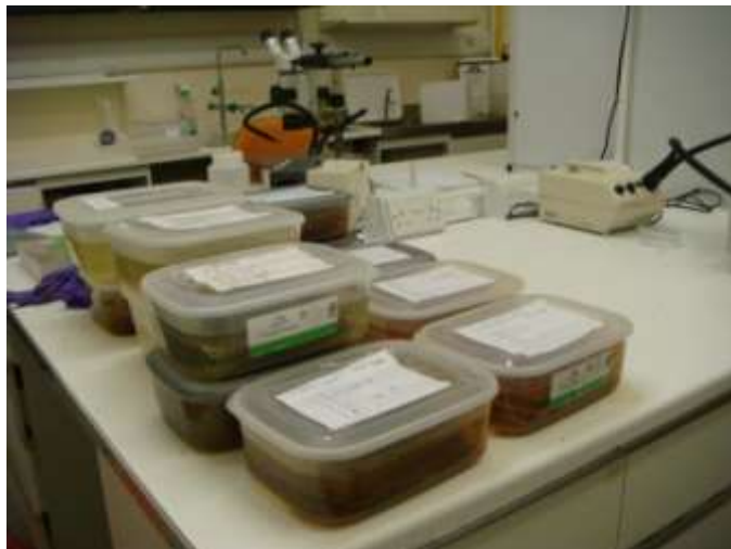
Plate 7. The short term panels are collected in 20 litre plastic containers and preserved in 70% ethanol.
