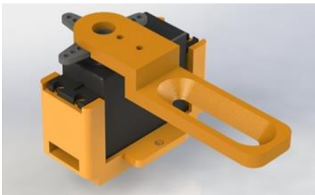
Fig. 5. Servo Mount with interface paddle in position.
