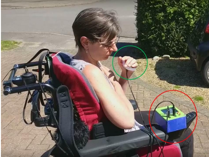
Fig. 10. The joystick manipulator (circled red) mounted on a powered wheelchair for final field testing, with the hand band mounted on the palm (circled green).
