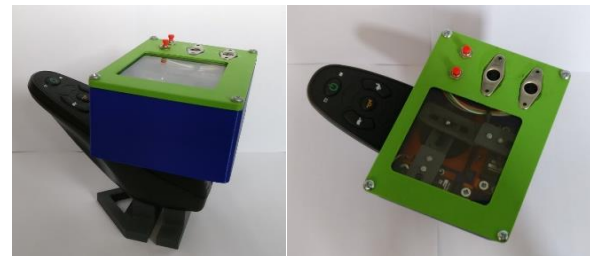
Fig. 3 The joystick control unit mounted on the test joystick jig.
