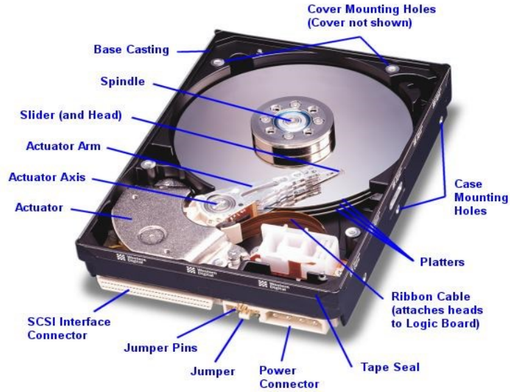
Figure 1.3: Hard disk drive components (Craig, 2007).
