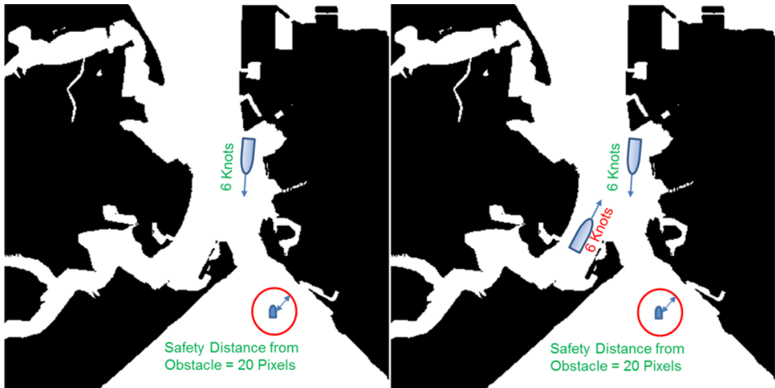
FIGURE 4.13: Binary map of the simulation area (Portsmouth harbour) showing velocity and direction of moving obstacles. In this study, 20 pixels has been chosen as the safety distance around an USV.
