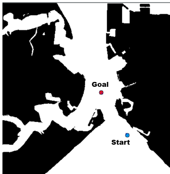
FIGURE 4.12: Binary map with start and goal states for simulating A* approach under static and partially dynamic environment
