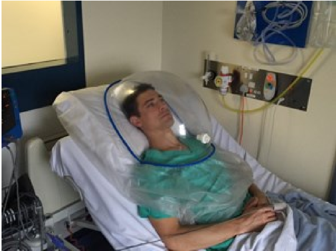
Figure 3 The GEM indirect calorimeter gas collection hood.
