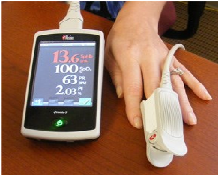
Figure 10 The Pronto-7 pulse co-oximeter
