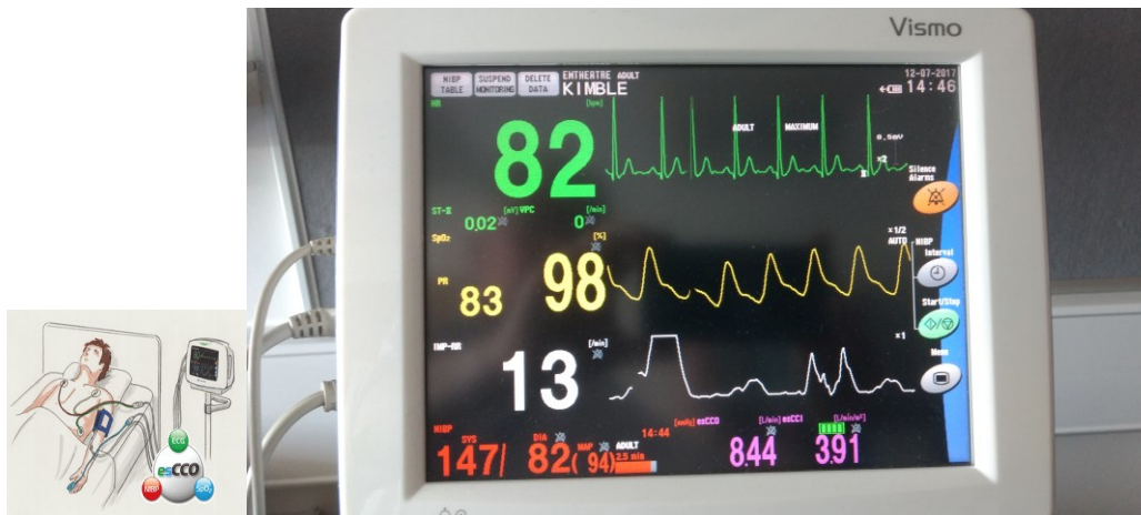
Figure 9 The esCCO cardiac output monitor
