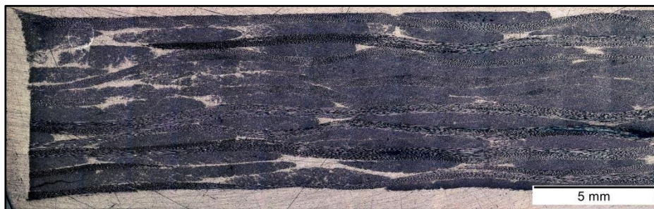
Fig. 5.4: Microscope picture of the crimp angle
