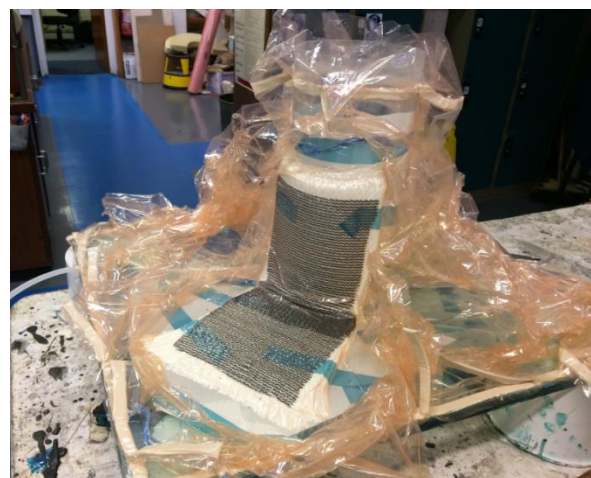
Fig. 4.13: The vacuum infusion process of the experiments
