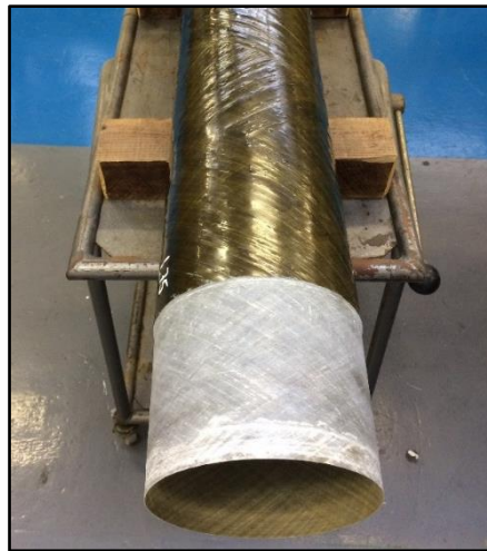
Fig. 4.25: Chamfering the composite pipe
