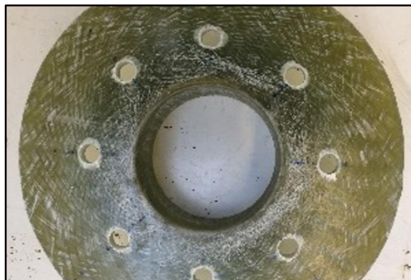
Fig. 4.15: Flange without dry fabric on the face
