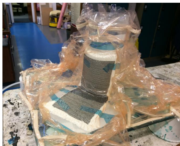
Fig. 4.13: The vacuum infusion process of the experiments
