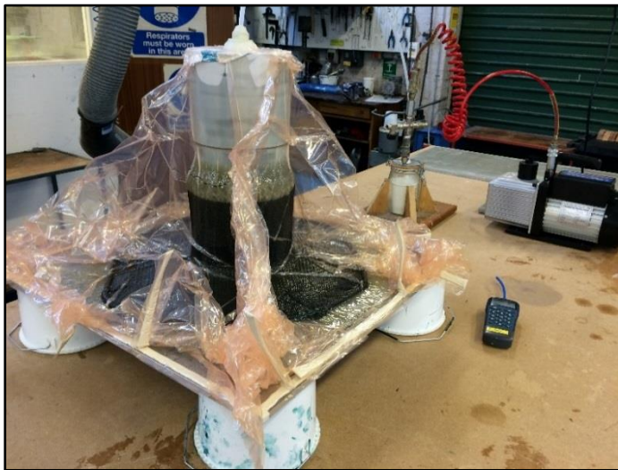
Fig. 4.8: Bagging and resin infusion
