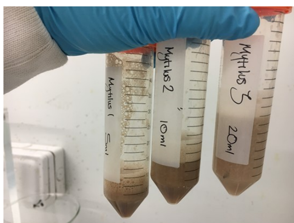
Figure 2.19. Whole mussel tissue homogenised in different volumes of DI water (5, 10, 20 mL).
