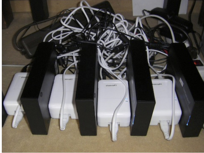
Figure 6.2: Set of Sheeva Plugs with Harddrive and Network connections
