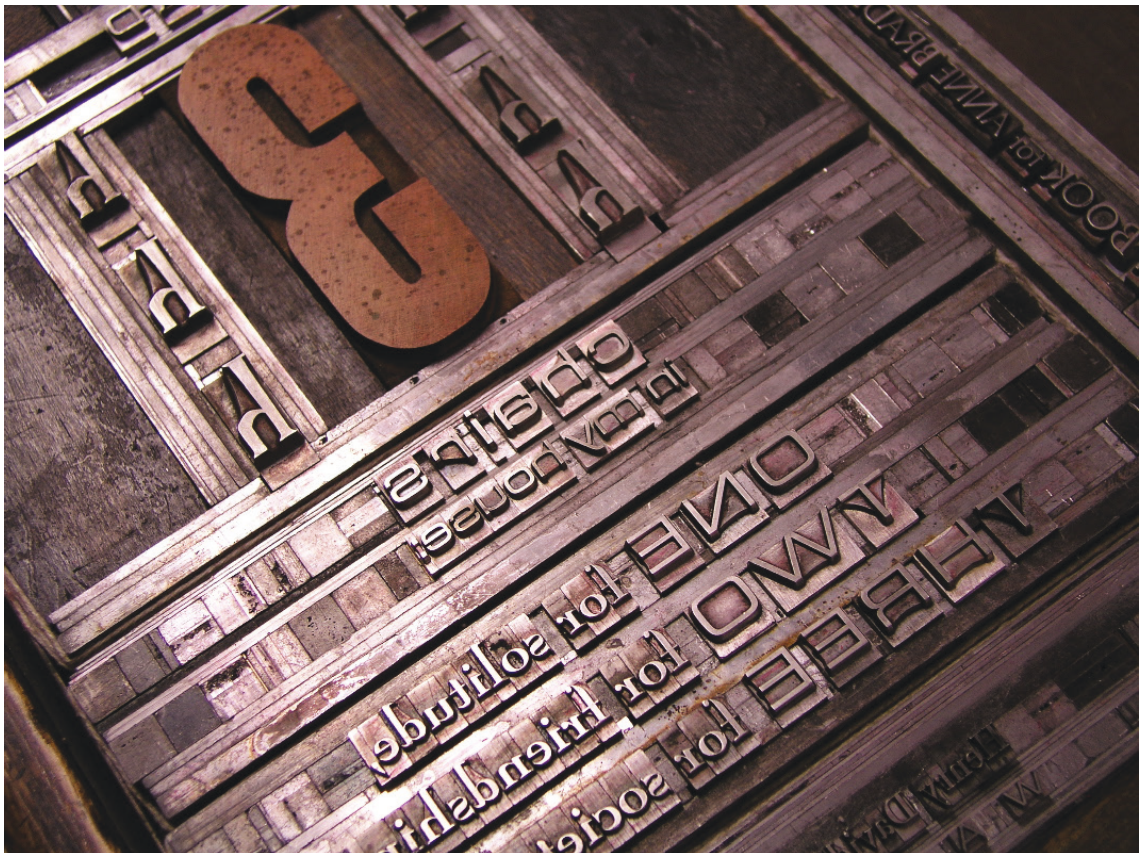
Figure 43. Hot type press composer ready to print showing the leading between the letters. Retrieved March 25, 2018 from: http://www.thewindowpanepress.com/
