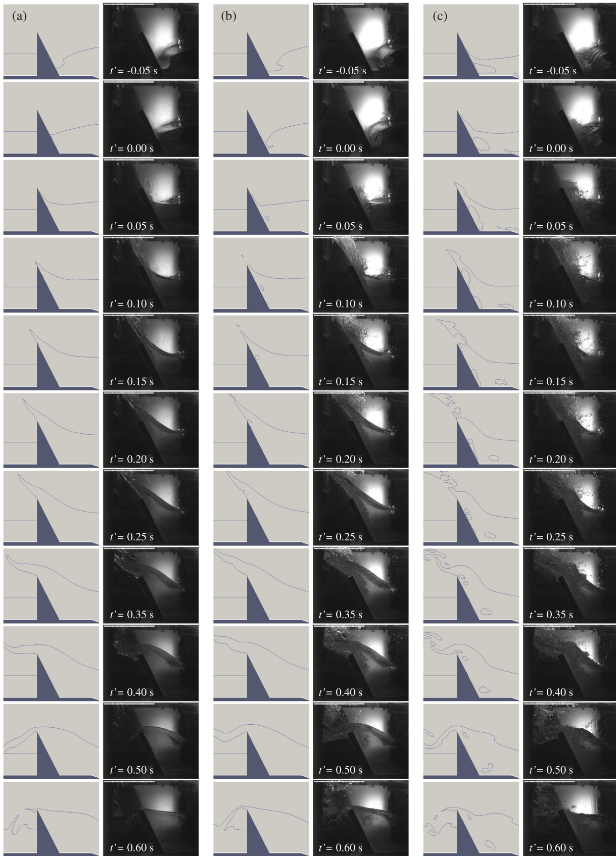
Figure 5 Comparison of numerical model output and video frame sequence for (a) steep-fronted wave; (b) plunging wave; and (c) broken wave overtopping of 150 mm freeboard wall
