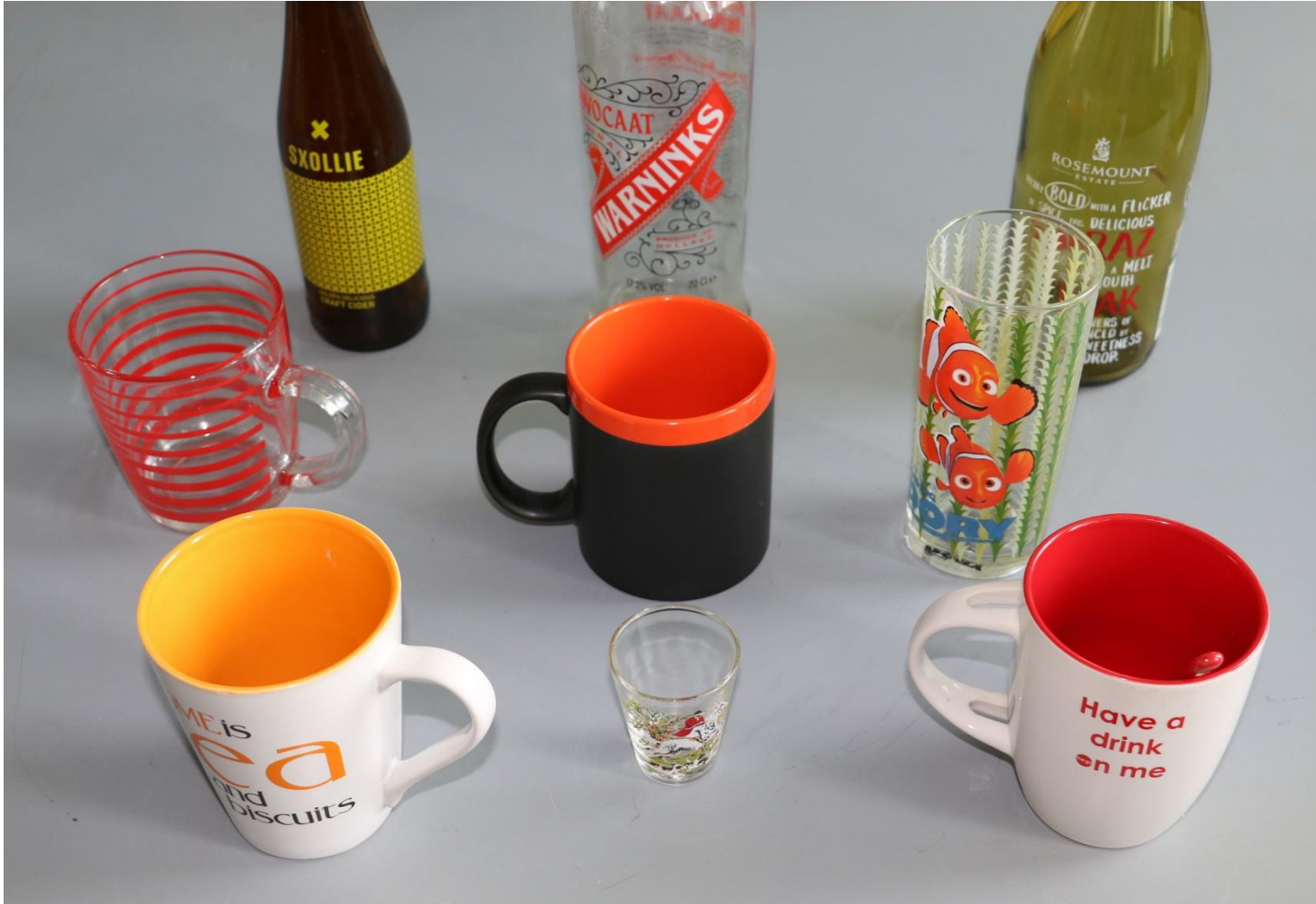
Figure 3: A selection of Cd-positive ceramic mugs and decorated drinking glasses and bottles analysed as part of the present study.
