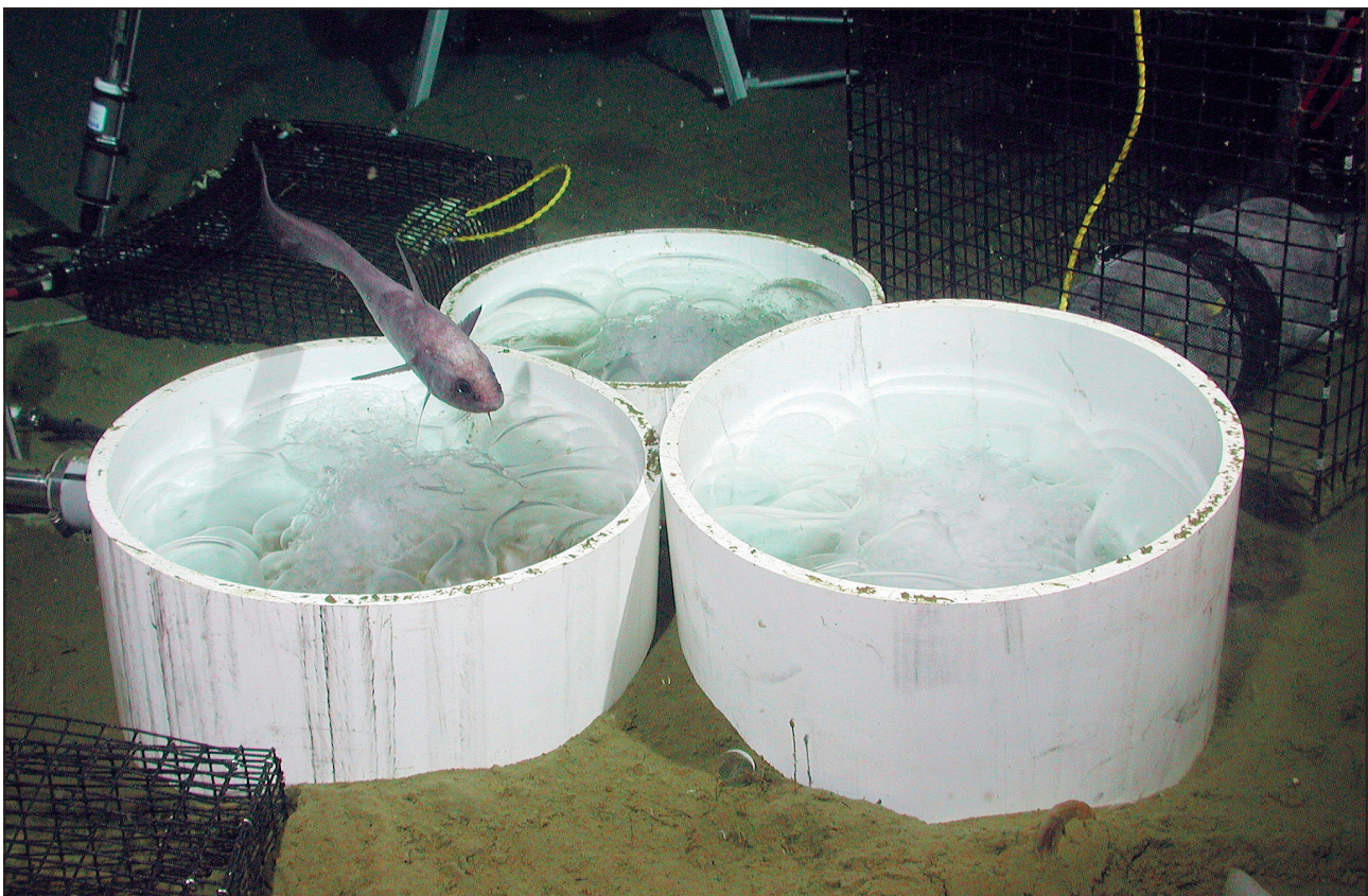
Figure 8.2 Photograph of manipulative deep-sea experiment to evaluate the response of deep-sea organisms to low pH / high \text{p}(\text{CO}_2) . Liquid \text{CO}_2 ( \sim 60 l) was released into PVC tubes ( \sim 45 cm diameter) placed on the seafloor at 3600 m depth off central California. The liquid \text{CO}_2 dissolved into seawater, producing a high \text{CO}_2 , low pH plume that drifted over the seabed and organisms in the sediment or held in cages at different distances from the \text{CO}_2 pools (photo credit: J.P. Barry).
