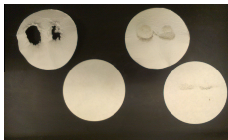
Fig. 5. Aspect of smears after being rubbed on 10 cm of concrete; top: paper filters; down: glass fiber disks; left: wet; right: dry.
