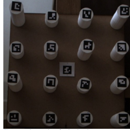
Figure 7. A template for in-depth measurement with 16 targets at different heights.
