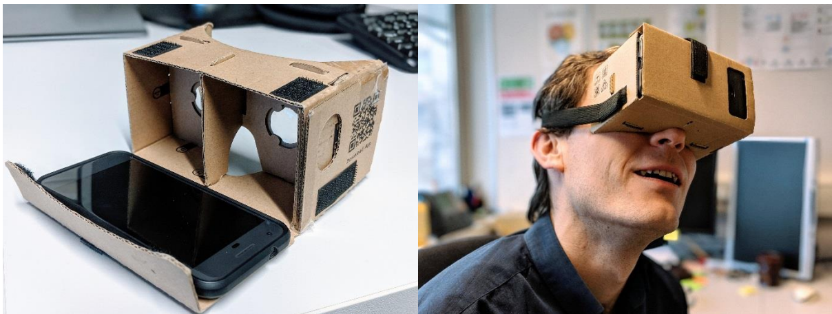
Fig 3. (Left) Shows how a mobile phone is placed as the display for Google Cardboard head mounted display. (Right) Shows the placement of the Google Cardboard display in use.
