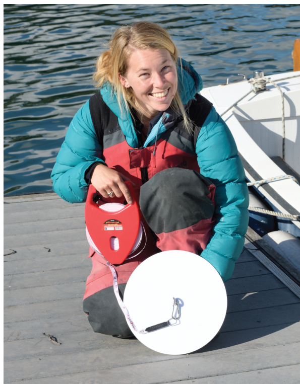
Fig 1. Seafarer citizen scientist and yachtswoman susie goodall with a 30 cm diameter Secchi Disk and Fibreglass tape measure.
