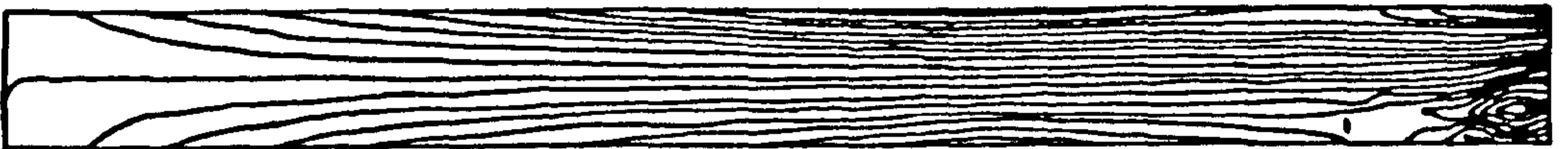
y-stress contours from 189 to -210 in steps of 21
