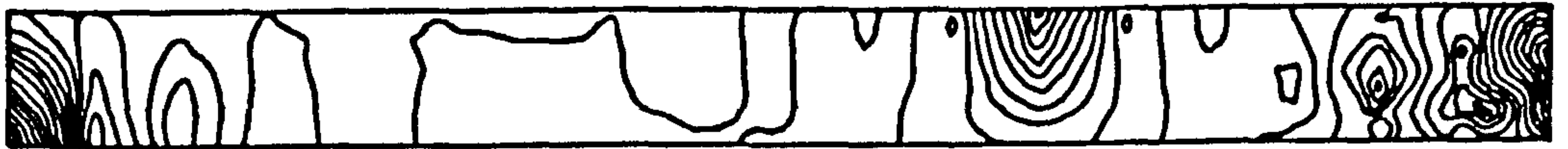
x-stress contours from 22 to -34 in steps of 2
