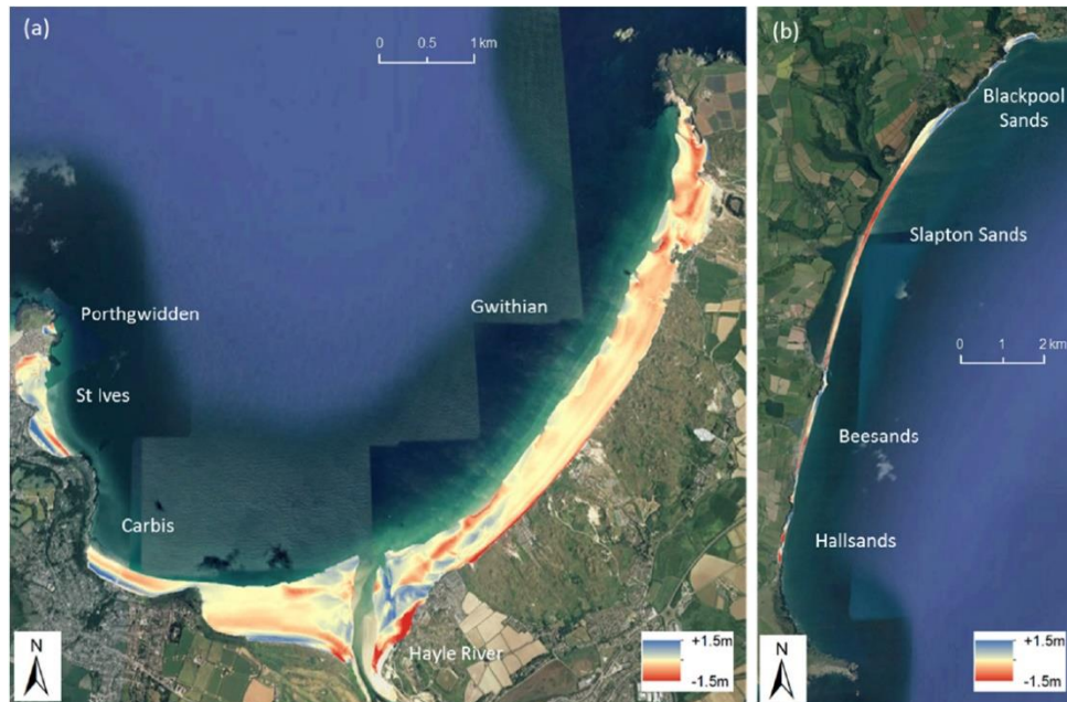
Figure 2.13: DoDs obtained from LiDAR data along (a) St. Ives Bay beach surveyed in April 2012 and April 2014, and (b) Start Bay surveyed in April 2012 and April 2014, illustrating spatial change in beach response and sediment connectivity between adjacent beaches at a local scale. Their location along the south west coast of England is presented in Fig. 2.12. Erosion is coloured in red whereas accretion is coloured in blue.
