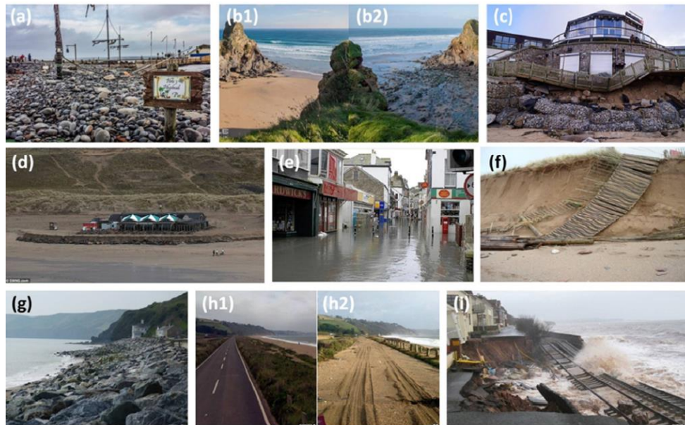
Figure 2.1: Pictorial overview of storm impacts during the 2013/14 winter along the coast of south west England (same site numbering system as in Figure 2.2). (a) The gravel barrier at Westward Ho! #19 experienced overwash (photo: Richard Murgatroyd). (b1) before; (b2) after) Large quantities of sand were removed from Whipsiderry beach #39, exposing the underlying rocky shore platform (photo: Mike Searle). (c) The seawall below Fistral Blu bar in Newquay #41 collapsed and causing damage to property (photo: Richard Murgatroyd). (d) The Watering Hole in Perranporth #46 required human interventions to protect the restaurant (photo from Mail Online, SWNS). (e) The coastal town of Looe #100 was flooded a number of times (photo: Nic Randall). (f) The coastal dunes at Thurlestone #119 experienced more than 5 m of erosion (photo: National Trust Southwest). (g) At the end of the winter, the beach in front of the seawall at Beesands #123 had completely disappeared. (h1) before; (h2) after) The road that runs along the gravel barrier of Slapton Sands #124 became covered with gravel due to overwash (photo from BBC News, Press Association). (i) The most costly damage occurred to the London-Penzance railway line at Dawlish #139 (photo from BBC News, Press Association).
