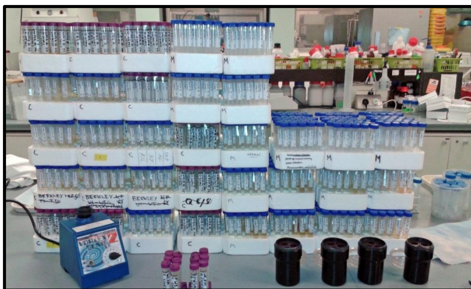
Plate 4.1: Falcon tubes (15 mL) containing mixed acid extractants following processing of soil samples collected in the crop and margin regions of Miscanthus x giganteus , willow short-rotation coppice and their respective cereal controls. Extractant solutions subsequently processed using ICP-OES for element analysis.
