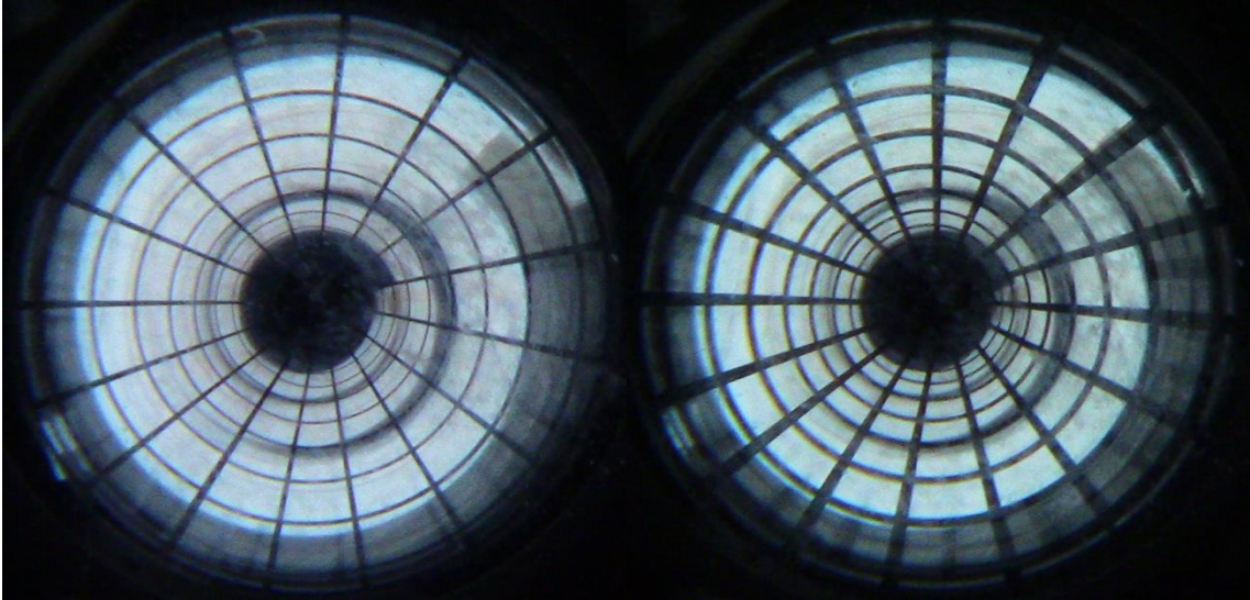
Figure 2.17: The appearance of OFTA mire 2 [1 mm (thin lines) and 2 mm (thicker lines) mire thickness] seen on steel ball.
