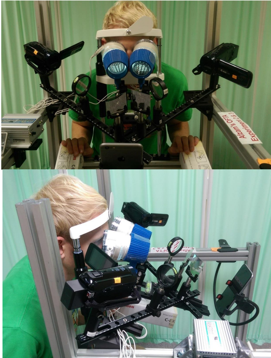
Figure 5.8: Participant's position for the reading task measurement. Note the reading material was being held by a holder.
