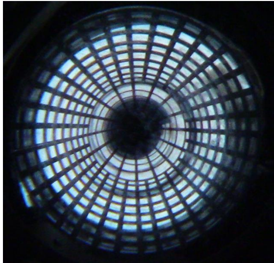
Figure 2.21: The appearance of OFTA mire 4 (2 mm mire thickness) seen on steel ball.
