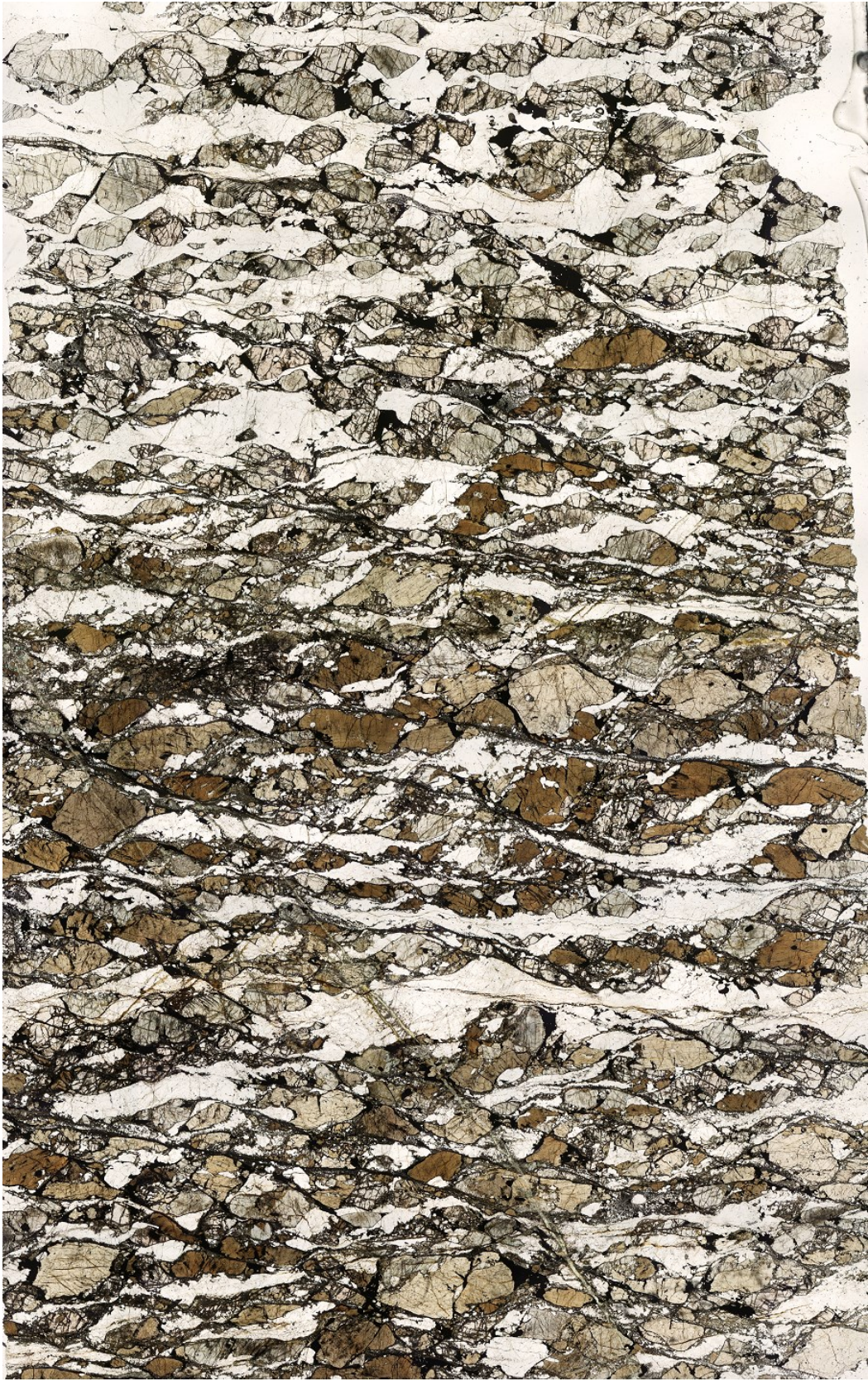
Sample F33: amphibole-poor metagabbro (upper portion), protomylonite; amphibole-rich metagabbro (lower portion), protomylonites. Scale bar 5mm.
