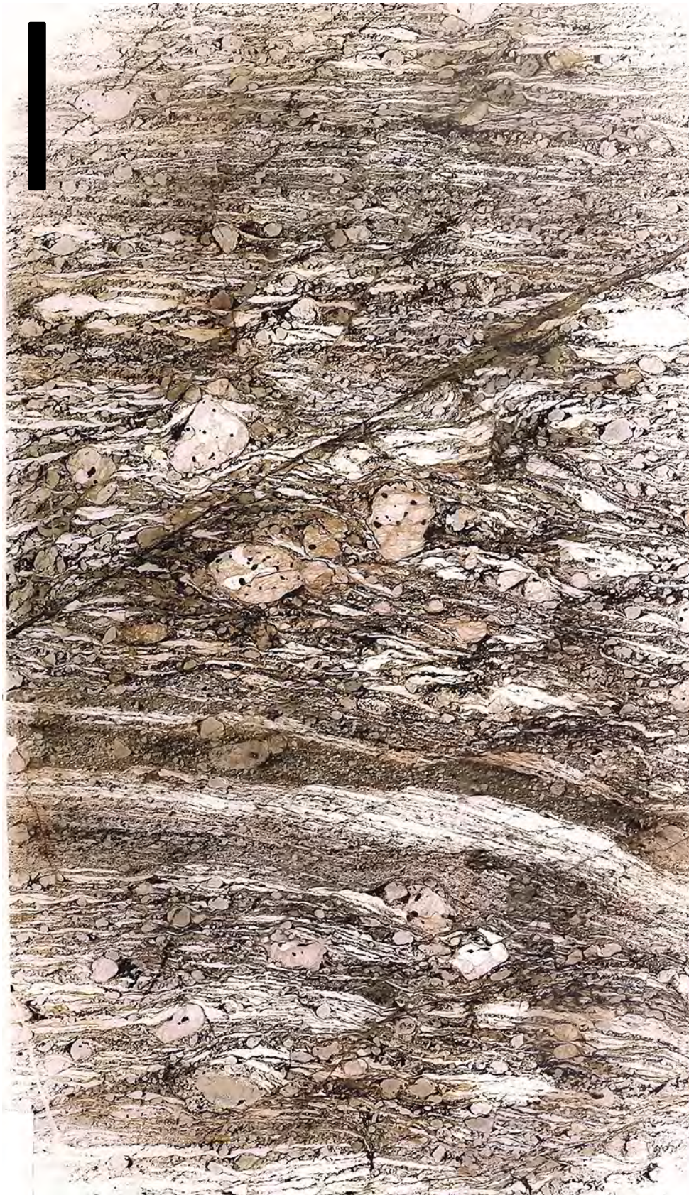
Sample F12A: Amphibole-poor metagabbro, mylonite. The sample has greenschist facies alteration, and the foliation is crosscut by greenschist facies fractures. This figure is a scan.
