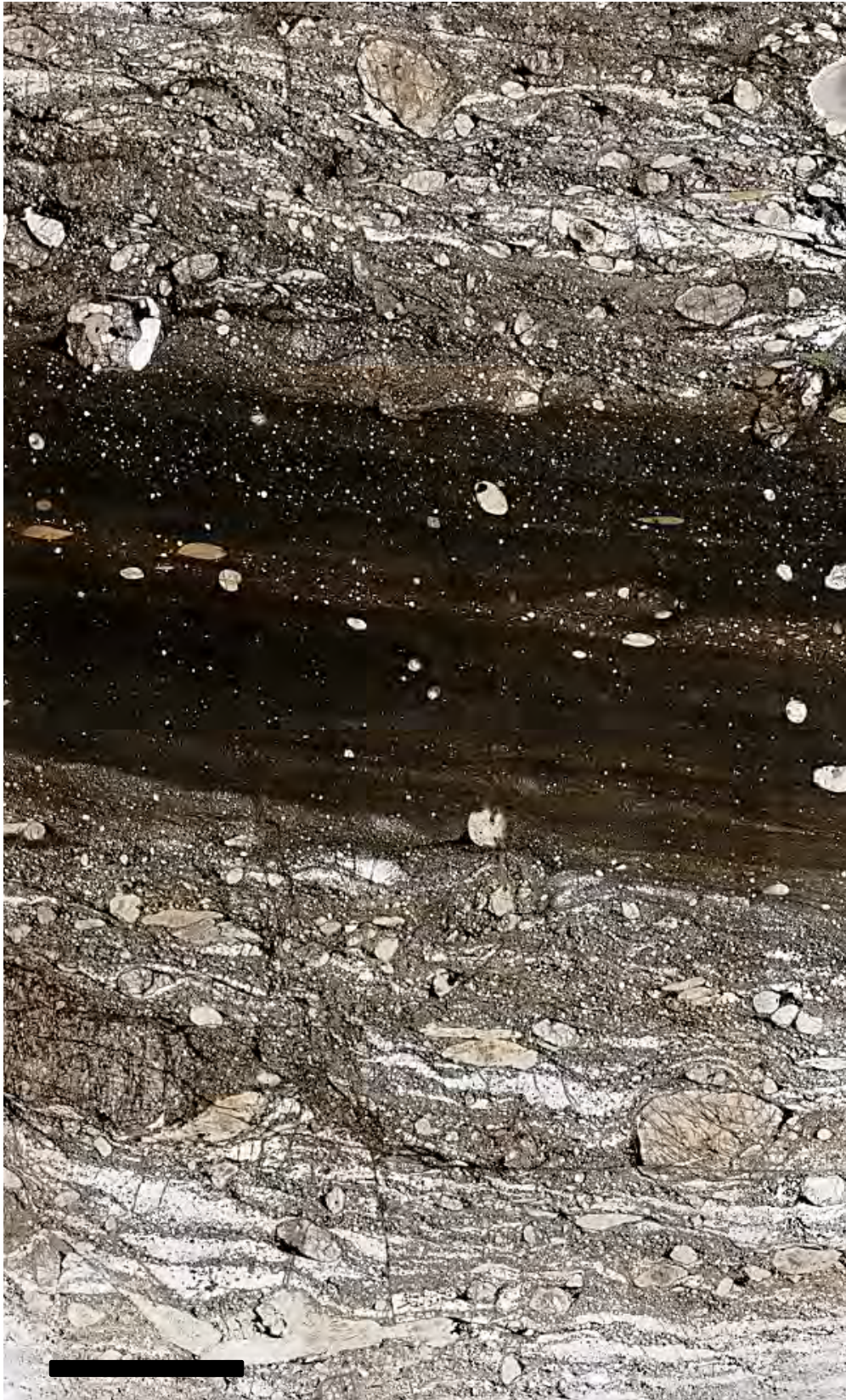
Sample F32C: Amphibole-poor metagabbro (upper and lower portions), mylonite. Amphibole-rich metagabbro (centre), ultramylonite. The sample has strong greenschist facies alteration overprint. Scale bar 5mm.
