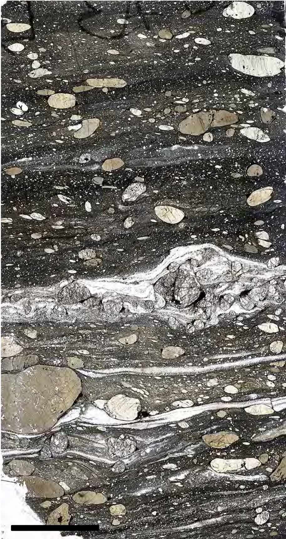
F10A3: amphibole-rich metagabbro, ultramylonite. Scale bar 5mm.
