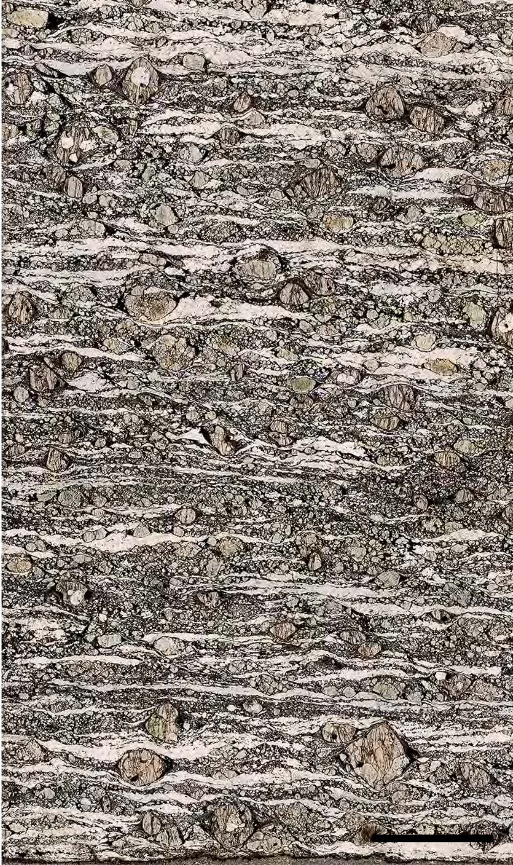
Sample F10B: Amphibole-poor metagabbro; mylonite. Scale bar 5mm.
