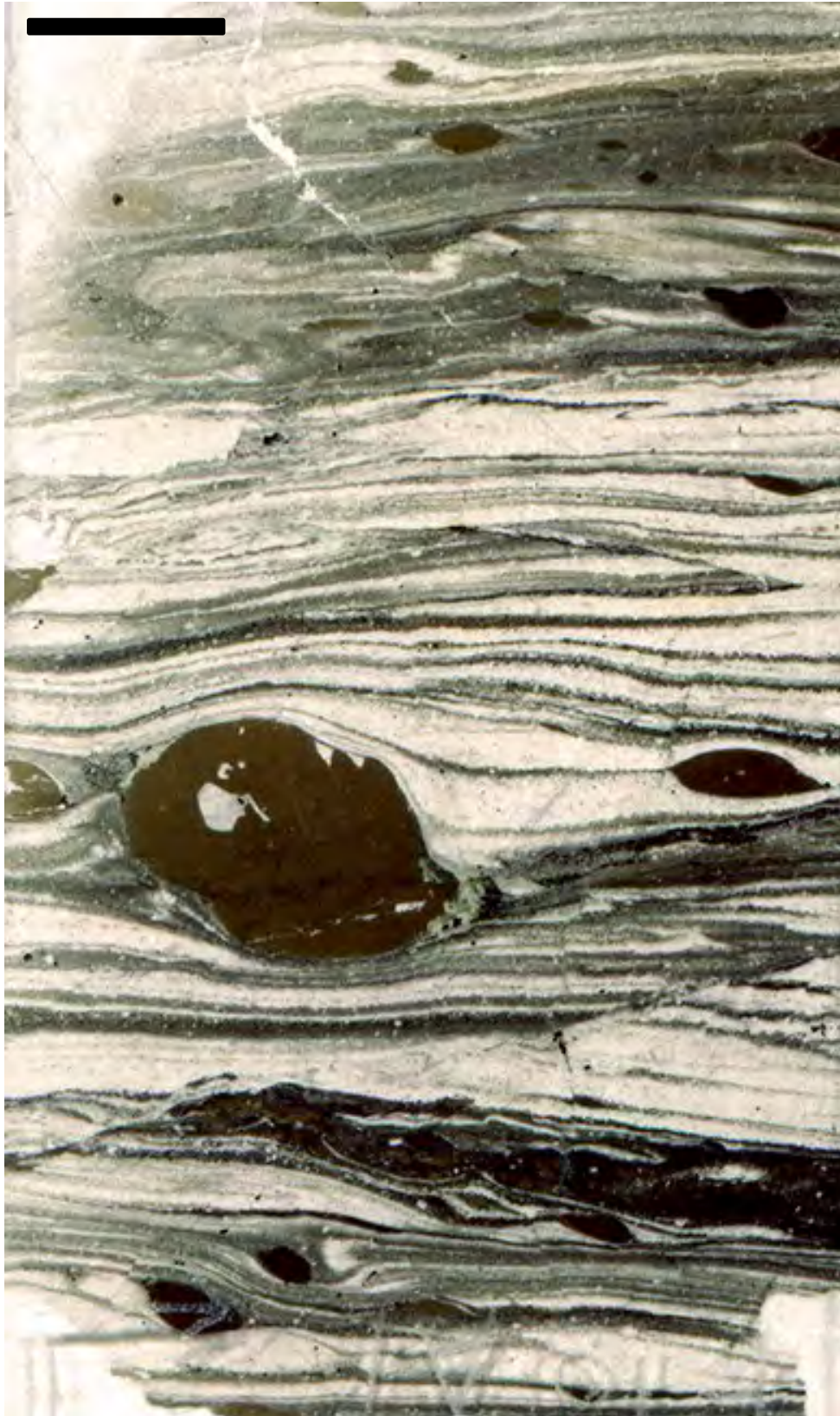
Sample F10A1: amphibole-rich ultramylonite, with amphibole-rich and plagioclase layers. This figure is a scan. Scale bar 5mm.
