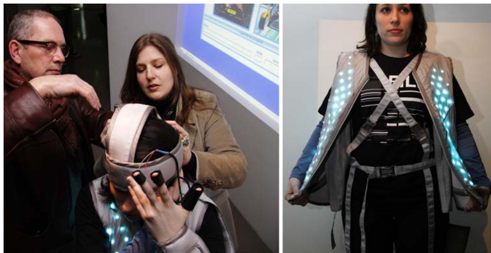
26. Figure: NeuroBodyGame by Rachel Zuanon & Geraldo Lima, 2010. Photo © Rodrigo Pessoa. NeuroBodyGame is a wearable computer embedded into a garment that allows the user to play games using their brain signals. (Figure 26)
