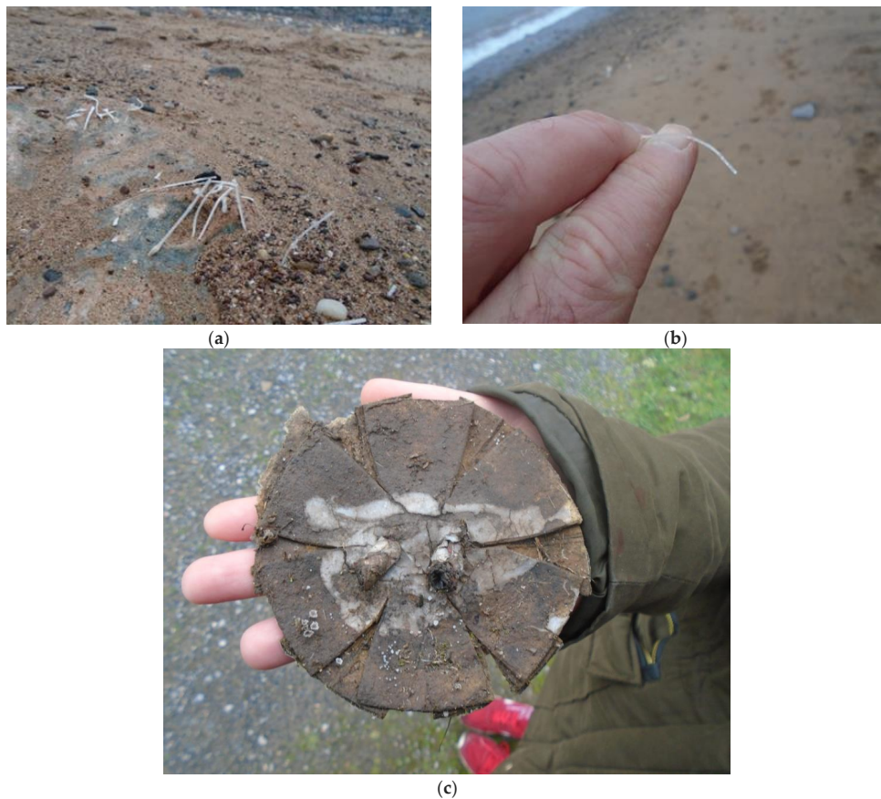
Figure 26. (a) Plastic strands from composite; (b) Plastic strand; (c) Funghi on filter.
