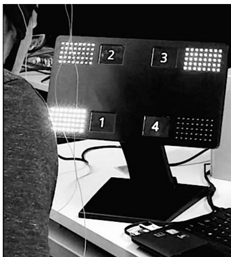
Figure 15: Photo of our new SSVEP stimuli device. In this photograph, the LCD screens are showing numbers, but in Activating Memory they display short musical phrases, such as the ones shown in Figure 16.
