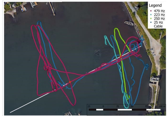
Figure 7 Experimental setup with testing cable and samples collected for different frequencies
