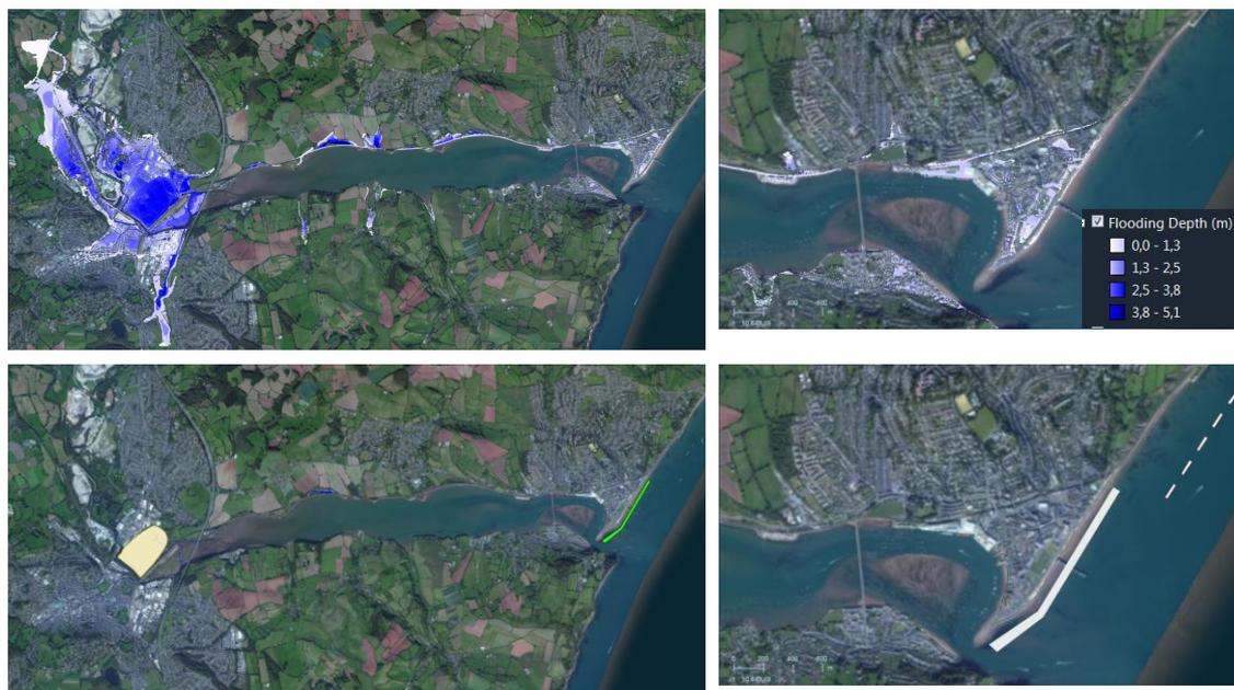
Figure 5. Flooding Depth: No mitigation options (up) vs All mitigations (down). Close up of detailed maps (right panels), for Mid-term conditions: 2050 yr, Tr 50 yrs.
