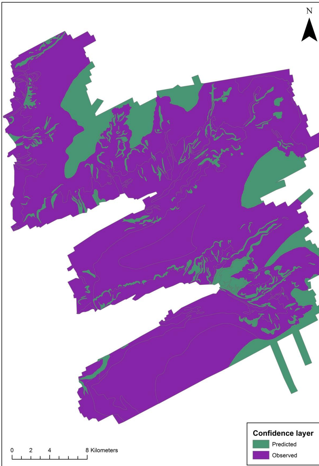
Fig 5.20: Confidence layer for biotope map of the SW Approaches. Those areas which had ground-truthing to inform the occurrence of biotopes within polygons are denoted in purple. Those polygons that lacked ground-truthing are in green.
