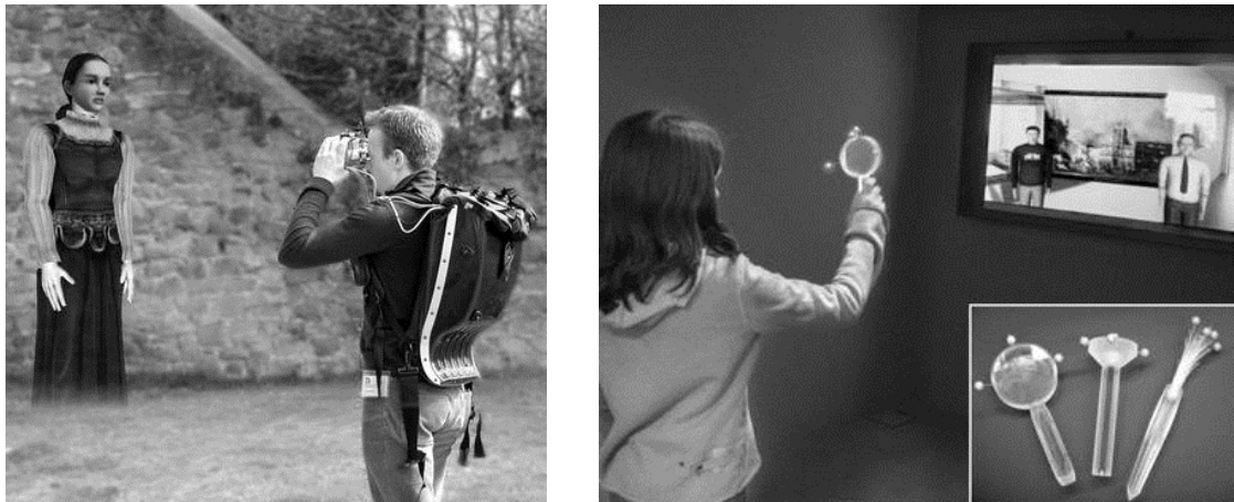
Fig. 2.7. Applying choices through special interfaces. Left: “GEIST” – in the Mobile-AR scenario, interaction occurs through finding ghosts by walking in real locations. Right: “art-E-fact” – video-tracked pointing gestures select parts of a painting, while special props define the meaning of the interaction (Spierling, 2005a).
