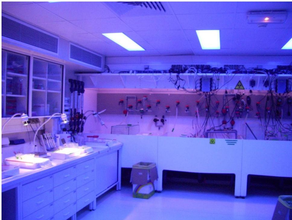
Figure 3-1: Experimental set-up for radionuclide exposure to adult zebrafish.
