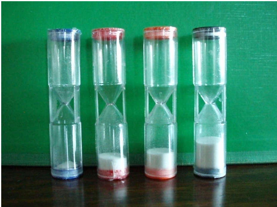
Figure 5.1 Sand-timers with delays of 30, 60, 90 and 120 seconds as used for the SCTs and SCTh delay discounting measures in Experiment 6.
