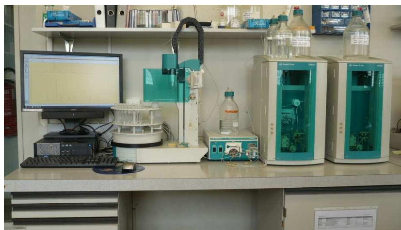
Figure 3-7: Ion chromatograph 882 Compact IC plus with autosampler (left), dialysis unit (middle) and the two 882 Compact IC plus units for anions (second from right) and cations (right).
