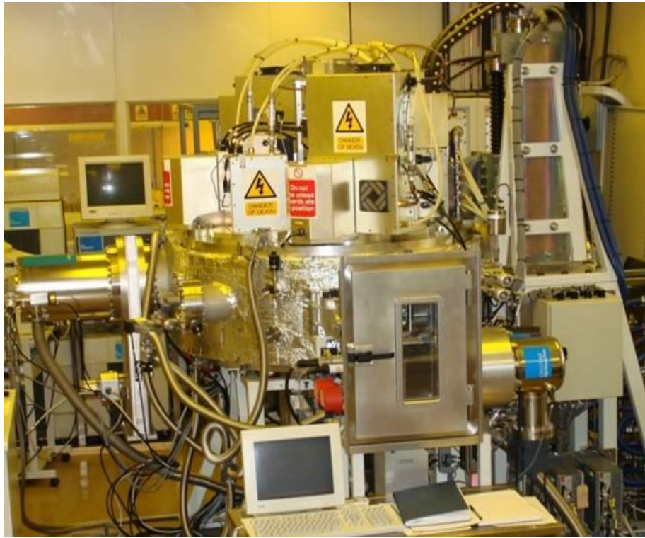
Fig. 3.1. Picture of Nordiko 9550 PVD sputtering system.
