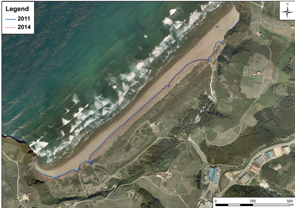
459 Figure 2: Dune toe recession at Xago.
