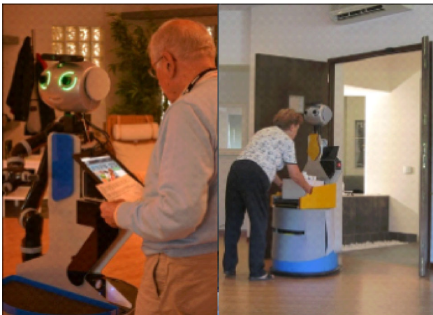
Fig. 4 Food delivery experimentation example: (left) After the user called the domestic robot via SUI, it turned to allow to detach the tablet and the user is reading the menu details via the GUI. (right) The user collects the goods from the condominium robot at the entrance door
