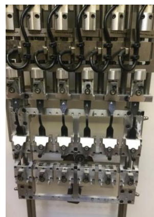
Fig. 1. Fatigue setup-up with samples at fully-relaxing conditions.
