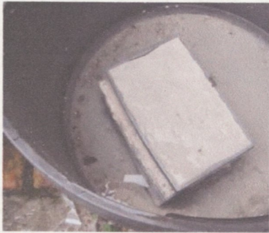
Figure 75 The test tank with three mortar samples installed. The white material at the bottom of the tank is a very thin layer of dust washed from the surface of the samples. It is not thought to have interfered with the trial results. The role played by the bottom of the tank, and the yard surface below it, is unclear and need further research.
